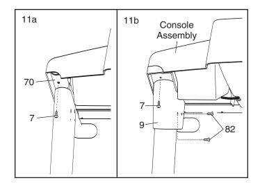
12 With the help of a second person, carefully lower the Uprights (85) to the position shown.
